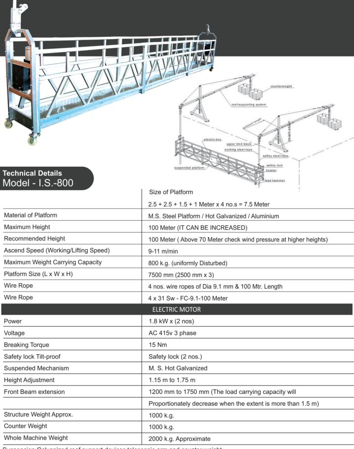
Suspension Galvanized roof support devices telescopic arm and counter weight
